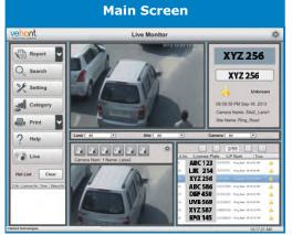
Main Screen display the image of the vehicles with their number plates. It stores vehicle's alpha-numeric number plate letters into text format and highlights any wanted/stolen hot-listed vehicle as per user define criteria.
